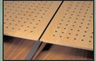
WoodTrends Elite is a genuine wood veneered ceiling panel system which installs easily into a standard 15/16" T-grid, leaving a 3/8" pencil line reveal between panels. This system is built on a MDF, chipboard, or plywood core with a veneer thickness of .6 mm. Unique compression spring technology allows for zero clearance above the grid and easy accessibility through any field panel. Standard sizes available are 24" x 24", 24" x 48" and 12" x 72". Available in 24 standard and 40 custom veneers.
