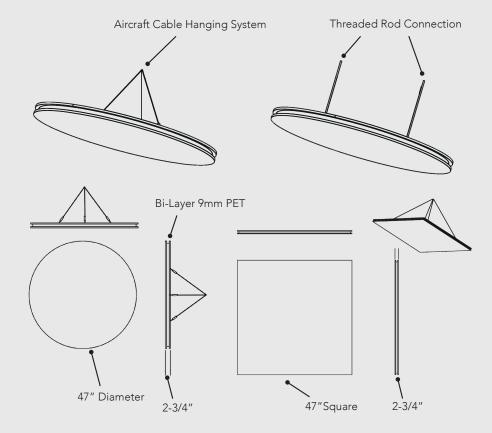
The aircraft cable method has two options; Multiple strands to the deck or a single strand to the deck with a sputnick hardware option.
